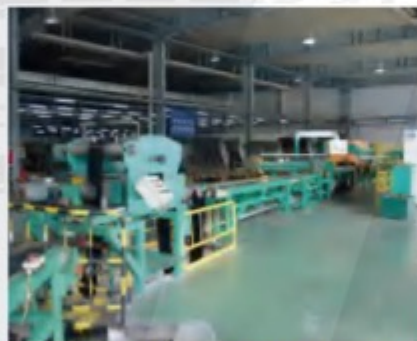
4. Small angle steel cord cutting line of Slovakia
