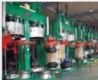
6. Steel-belted radial tyre hydraulic dual-mould curing press
