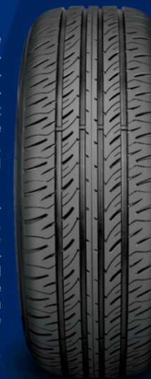
Excellent wet and grip performance, the four longitudinal grooves makes outstanding drainage performance and effectively prevent tires from slipping sideways in rainy days. The central straight rib and the lateral fine grooves make the tire more stable when driving at highway, which make excellent acceleration and braking.
